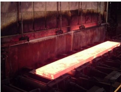
Hot Steel Slab Exiting the Furnace
