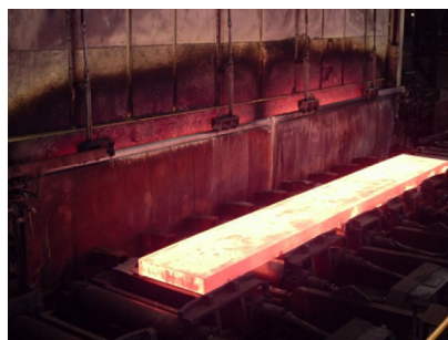
Hot Slab on top of Discharge Table Rolls
