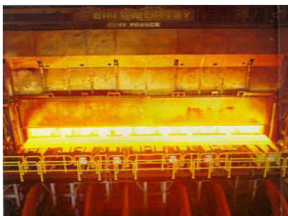
HSM Walking Beam Furnace
